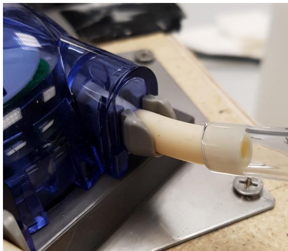
Figure 9: Pressure-fit vinyl tubing on peristaltic pump tubing (Pharma BPT).
